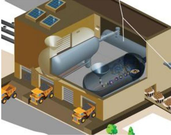
Bixby Energy Systems Inc. is trying to clean up the coal industry's smudged image by superheating coal in a closed-loop system (above) and creating synthetic natural gas to fire electric power plants (see pipeline at back right corner of plant). Founded in 2001, Bixby Energy Systems is headed by Robert Walker, who in a past corporate life founded Select Comfort Corp. The company just sold five Bixby Model 625 units to the city of Shanxi, China. (Graphic supplied by Bixby Energy)
